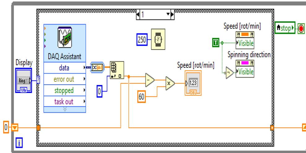
Fig.8. The part of the block diagram used for display speed of rotation
