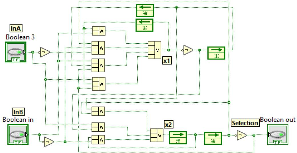
Fig.7. The logic configuration for spinning direction identification
